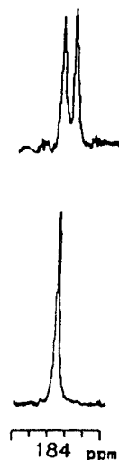
Figure 5 Effect of N-100 on the ^{13}\text{C} -NMR spectra of carboxylic carbons of DBTDL in \text{CDCl}_3 solution. Bottom: original spectrum of DBTDL. Top: spectrum obtained after addition of N-100.
